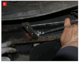
NOTE: Before fitting the Scorpion system the rear mounting point needs re-locating
